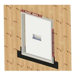
**6)** Fasten the window using pan head screws. For white or adobe product, use a screw in every other nail flange hole. For painted or carbon series product, use a screw in every flange hole. Check level and plumb intermittently during this step.
