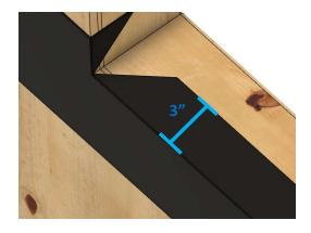
2) Install another strip of flashing tape of the same width on the sill, flush with the interior face of the opening. Fold the ends of the flashing tape up both sides 9".
