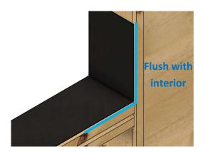
**3)** Use 1/4" to 1/32" shims to level the sill. This ensures that the window will operate smoothly and expel water as intended.
