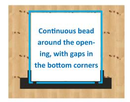
**5)** From the exterior, place the window into the opening. Center the window and ensure the nail flange makes contact with the caulk on all sides. The caulk should spread out when compressed, and appear from the holes in the nail flange. Check that the window is level and plumb.
