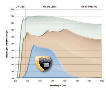
What makes multi-layer LoE³-340 different is its ability to handle each portion of the solar spectrum differently.
